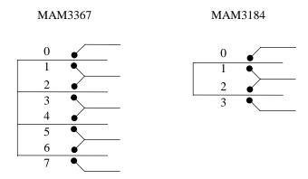
Figure 1.3 Disk/head configuration
